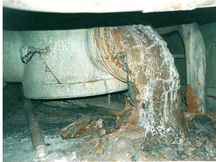
4 Unit of ChNPP– solidified fuel-containing substance from steam-relief valve
