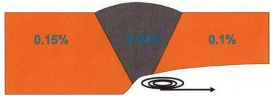
Degradation on weld root and downstream component – disturbance near the weld
