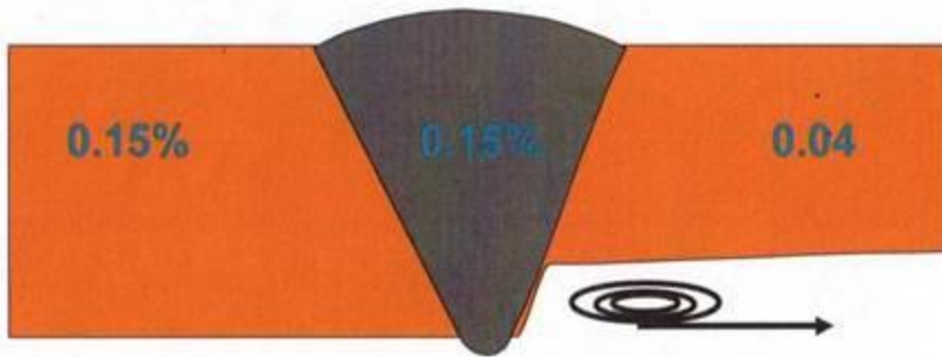
No degradation on weld root disturbance near the weld (penetration)
